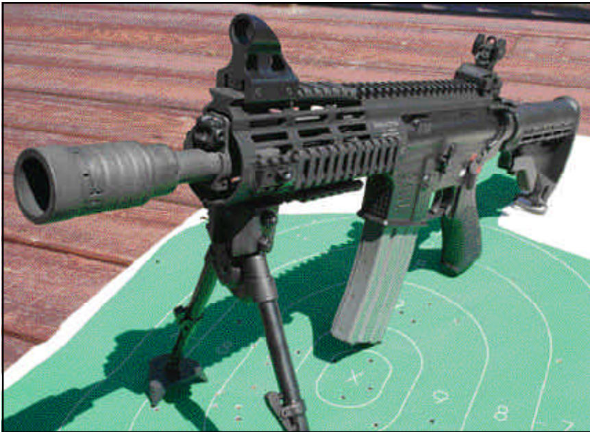
Above: The 9.25-inch system combined with the "Krink" style muzzle brake and any of the rate-reducing buffer systems tested proved to be extremely controllable and effective even under full automatic fire.
