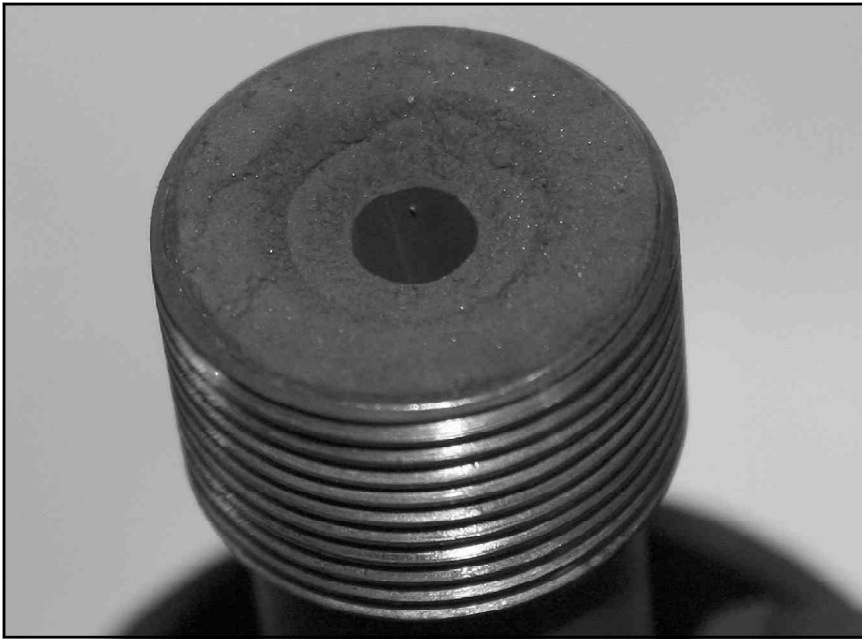
Above: The carbon on the muzzle area of the 9.25-inch barrel behind the “Krink” muzzle brake is obviously excessive from the endurance test.
