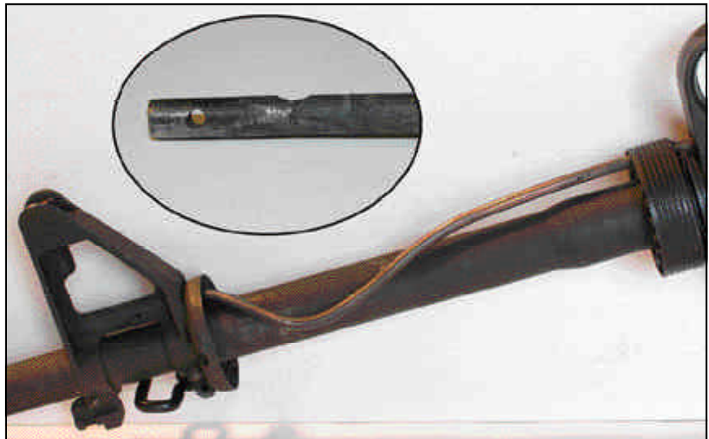
Above: Examples of potential problems with traditional gas tubes. This obvious failure happened during excessive firing at a very high rate of fire. There was a substantial amount of gas port erosion leading to the overheating. In the inset photo a gas tube can be seen having cracked to the point where gas would escape and no longer cycle the gun.
